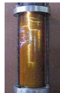
Figure 8. The "lightning" that occurs on a filter element is localized when it occurs.
