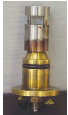
Figure 1. A valve stuck with lubricant varnish.
