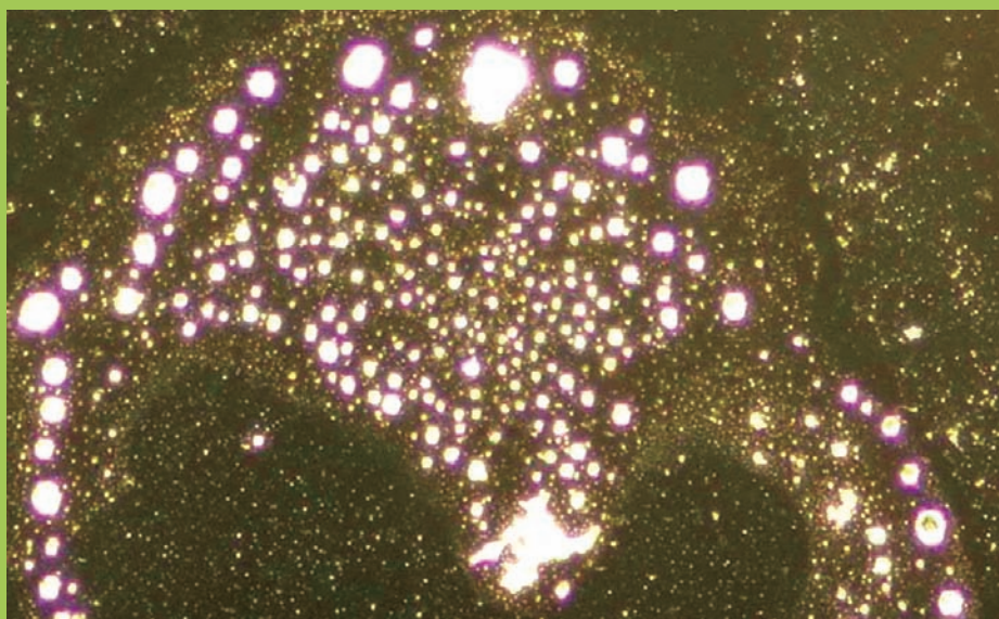
Figure 7. This microphotograph shows the fine balls of nylon produced by spark discharges of static electricity.
